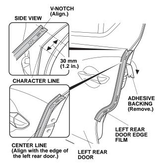
11. Align the center line on the left rear door edge film with the edge of the left rear door. While applying light pressure, carefully remove the adhesive backing, and attach the left rear door edge film to the left rear door. 12. Starting from the top and working downward, use the soft sleeve to smooth the left rear door edge film. Move the soft sleeve in one direction only.
