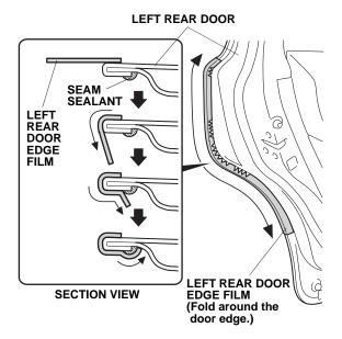
15. Using a shop towel, wipe the excess 3M protective tape application solution from the left rear door edge film. Allow the left rear door edge film to dry thoroughly.
