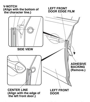
Align the center line on the left front door edge film with the edge of the left front door. While applying light pressure, carefully remove the adhesive backing, and attach the left front door edge film to the left front door. 5. Insert the applicator into the soft sleeve. Starting from the top and working downward, use the soft sleeve to smooth the left front door edge film. Move the soft sleeve in one direction only.
