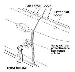
3. Open the left front door. Peel back about 50 mm (2.0 in.) of adhesive backing from the left front door edge film. Align the V-notch with the bottom of the character line on the left front door as shown.
