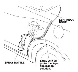
10. Open the left rear door. Peel back about 50 mm (2.0 in.) of adhesive backing from the left rear door edge film. Align the V-notch 30 mm (1.2 in.) above the character line on the upper part of the left rear door as shown.
